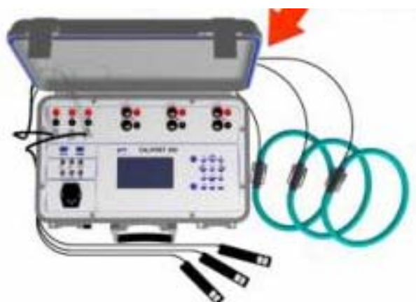
Example of a test set utilizing flexi CTs
